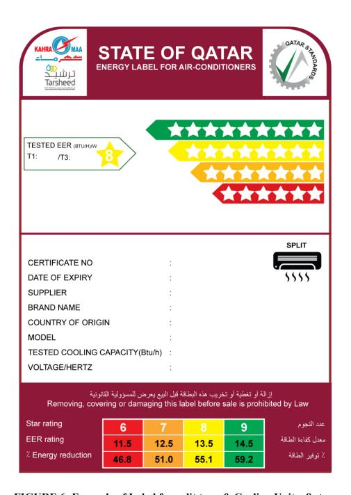
FIGURE 6: Example of Label for split type & Cooling Unit – 8 stars
