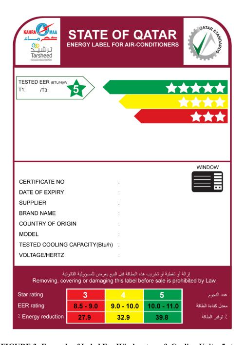
FIGURE 3: Example of Label For Window type & Cooling Unit – 5 stars
